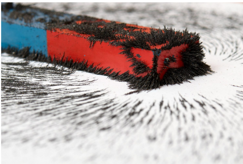
Iron filings line up along the field lines, showing the field pattern of a bar magnet
