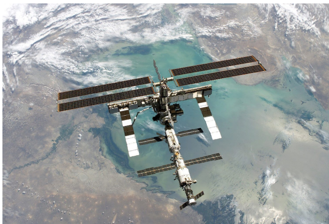
The ISS in orbit: orbital speed is the speed that keeps a satellite in free-fall circular motion
