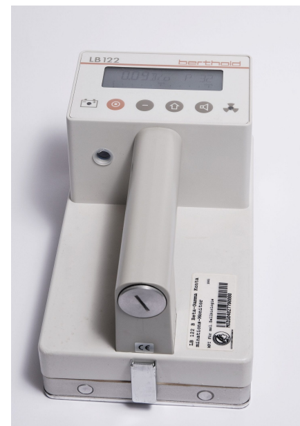
A portable Geiger counter detects ionising radiation and shows the count rate on its screen
