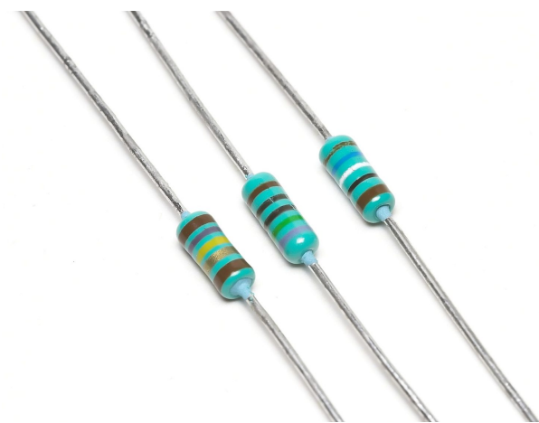
Real resistors: the coloured bands give each one's resistance in ohms
