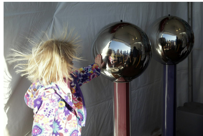
Every hair picks up the same charge from the dome, and like charges repel — so the hairs push apart
