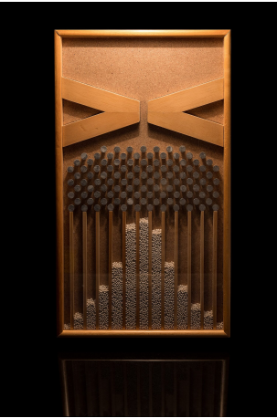
A Galton board shows how data piles up into a distribution.
