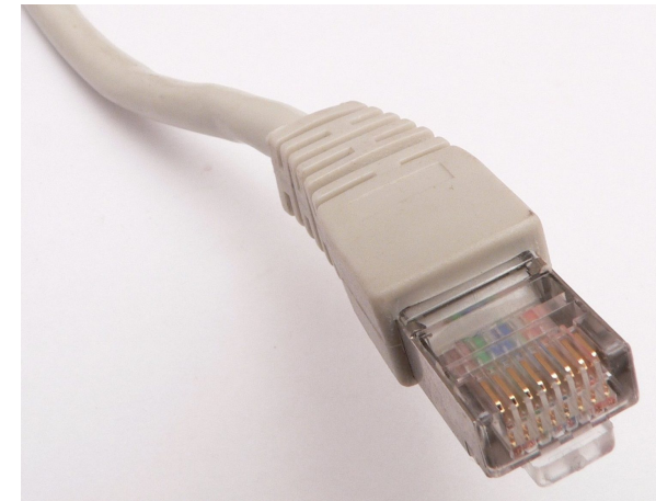
An Ethernet cable with an RJ45 plug, often used to carry data on a wired network
