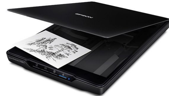
A flatbed scanner: it shines light across a page to copy it into the computer
