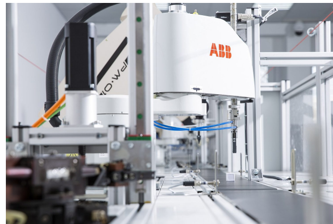
An industrial robot arm. It follows a program and can be reprogrammed to do a new job.
