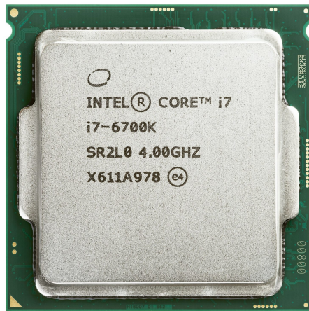
A central processing unit (CPU): the chip that processes data and runs the instructions
