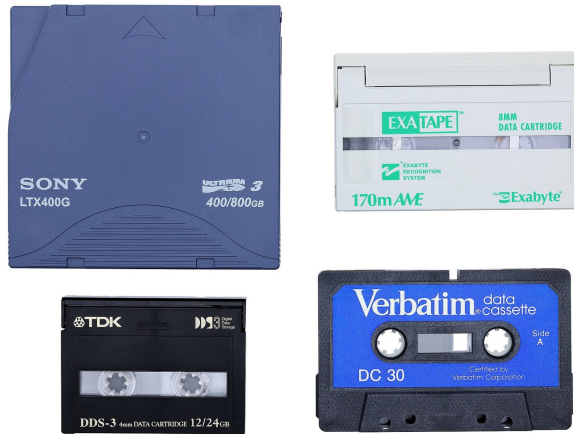
Magnetic tape stores data on a long magnetic strip; it is cheap for large backups
