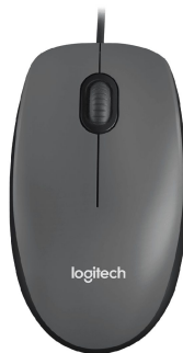
An optical mouse: a light and a sensor track its movement on the desk
