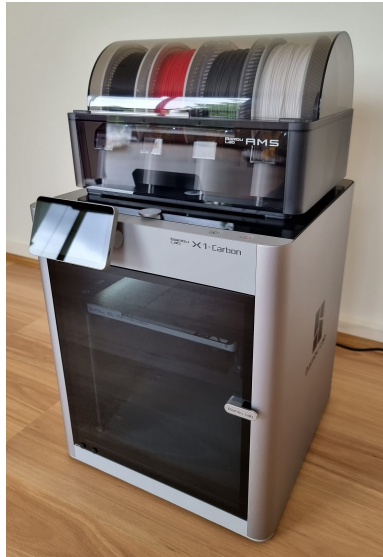
A 3D printer builds a solid object layer by layer
