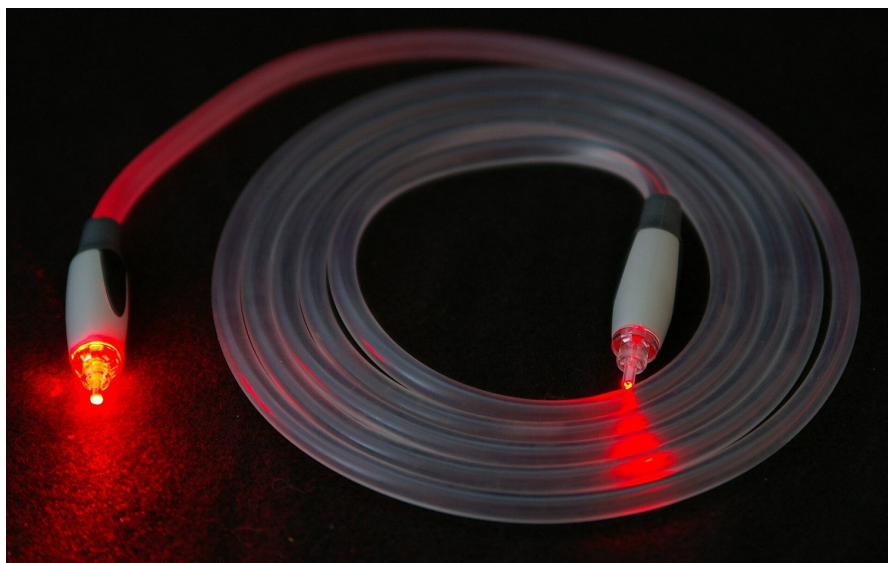
A fibre-optic cable carries data as pulses of light along thin glass fibres
