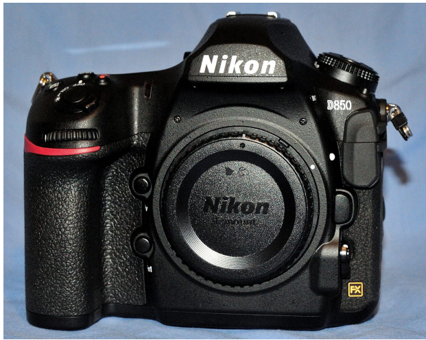
A digital camera: a lens focuses light onto a sensor that records the pixels
