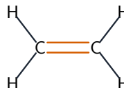
ethene \text{C}_2\text{H}_4 unsaturated: C=C double bond
