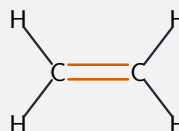
ethene \text{C}_2\text{H}_4 unsaturated: C=C double bond
