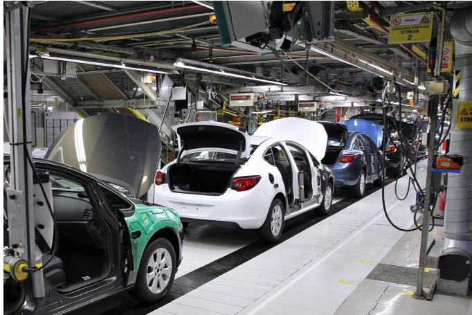
A car assembly line: making many identical products on a moving line
