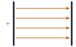
a) parallel plates (uniform field)
