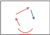
convection: hot fluid rises, cooler fluid sinks — a circulating current
