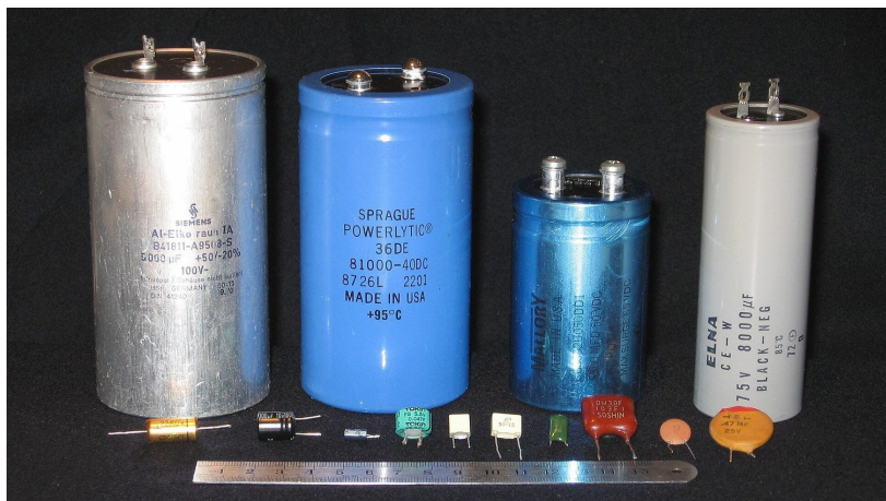
Assorted capacitors: devices that store charge and energy in an electric field between conductors
