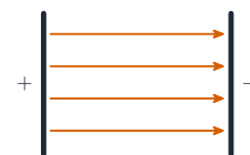
a) parallel plates (uniform field)
