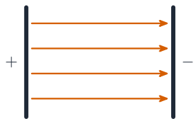
a) parallel plates (uniform field)
