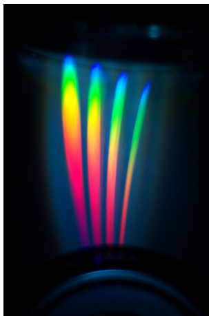
The fine tracks on a CD act as a diffraction grating, splitting white light into a spectrum
