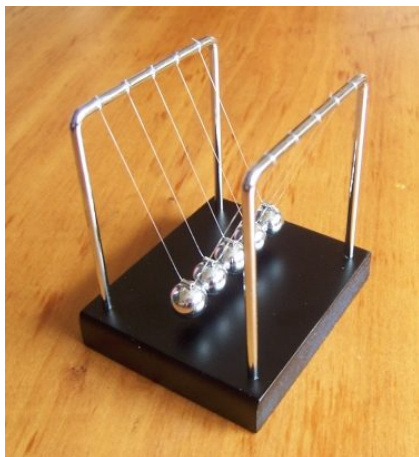
A Newton's cradle shows momentum and kinetic energy passing through a line of balls in a near-elastic collision
