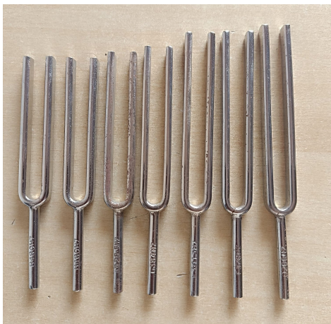
Tuning forks: a longer, heavier fork vibrates more slowly, giving a lower frequency
