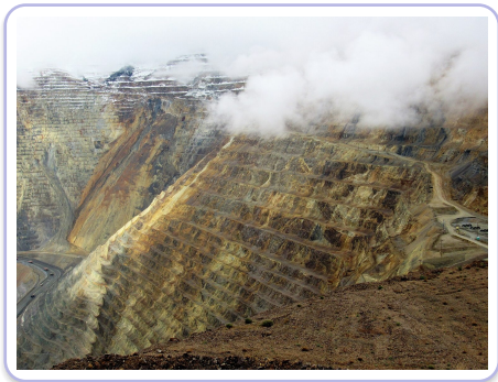
Benches cut ever wider and deeper to reach the ore
