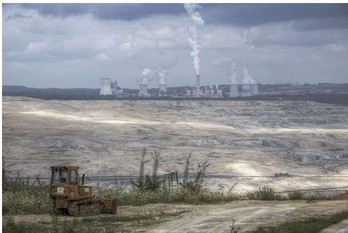
An open-pit lignite 褐煤 (brown coal) mine feeding the power station 发电站 behind it — the fuel is dug from the ground and burned on the spot
