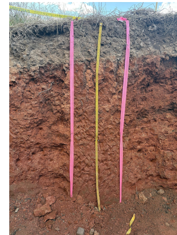
A pit dug through soil shows its horizons: dark organic topsoil on top, then paler mineral layers, over broken rock (tape for scale)
