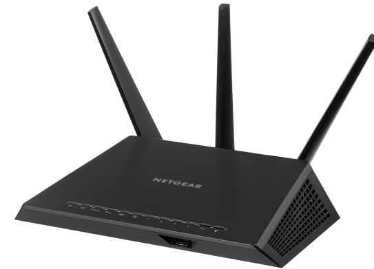
A Wi-Fi router: the local gateway that forwards packets toward the wider Internet
