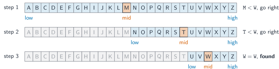
Binary search halves the range at each step (the list must be sorted)
