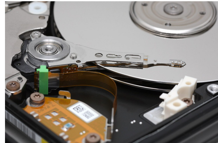
Hard-disk platters and head: data compressed and stored as magnetic patterns
