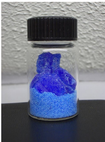
Blue copper(II) sulfate crystals grown from solution: a saturated solution left to evaporate deposits its dissolved solid back out as regular crystals
