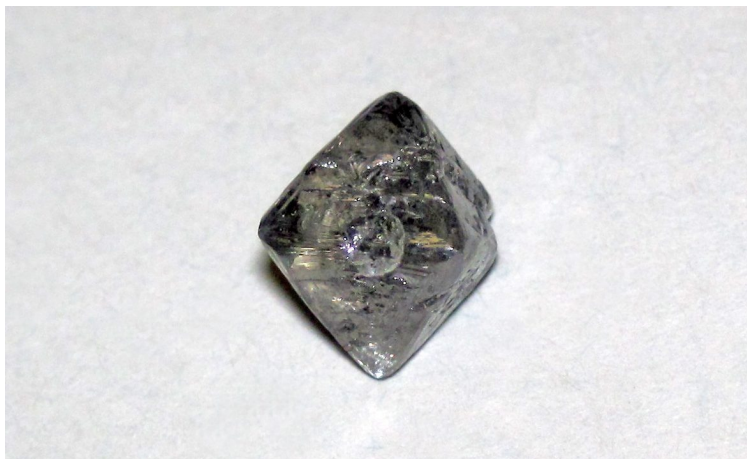
A diamond crystal: giant covalent networks explain extreme hardness and high melting points
