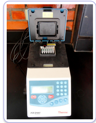
PCR: DNA replication run in a machine
