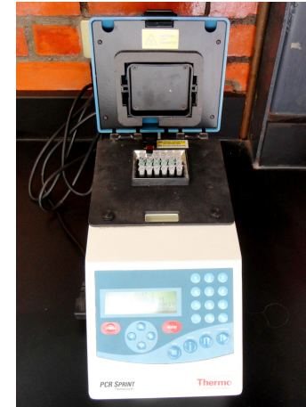
A thermal cycler repeatedly heats and cools samples to amplify DNA (PCR)
