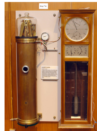
A pendulum clock keeps time using simple harmonic motion.
