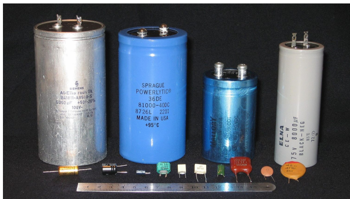
Real capacitors range from large electrolytic cans (high capacitance) down to tiny film and ceramic types – from pF up to mF
