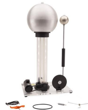
A Van de Graaff generator stores a large static charge on its metal dome, making a strong electric field around it
