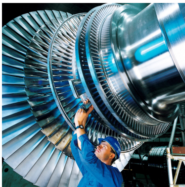
A steam turbine does work as expanding steam pushes its blades around.
