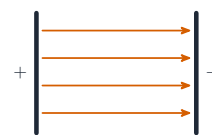
a) parallel plates (uniform field)
