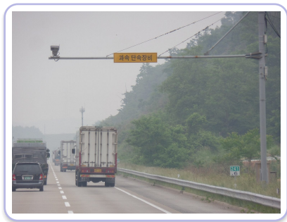
An average-speed camera times each car over a known distance
