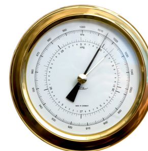
A precision aneroid barometer measures atmospheric pressure
