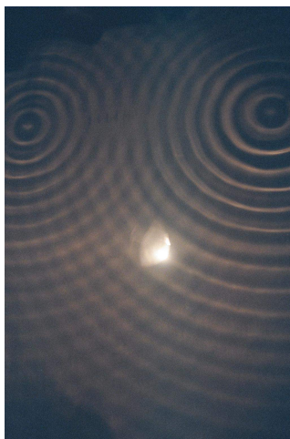
The same effect in a real ripple tank — two coherent sources give a steady interference pattern
