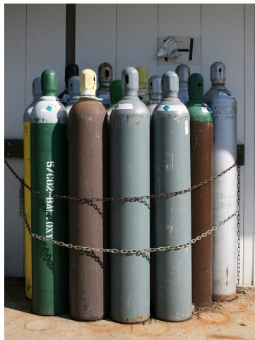
Compressed gas cylinders store a fixed mass of gas at high pressure.
