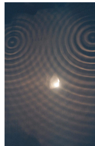
The same effect in a real ripple tank – two coherent sources give a steady interference pattern
