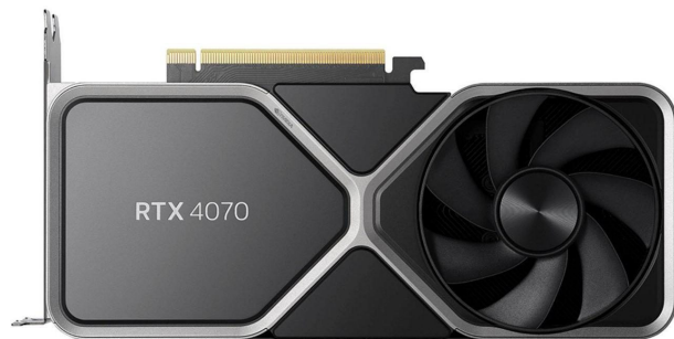
A graphics card: its GPU runs the same instruction on many data items at once (SIMD)
