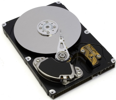
An opened hard disk: the actuator arm carries the read/write head over a platter
