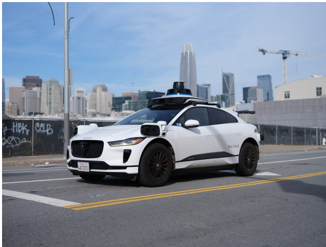
A self-driving car uses cameras and lidar sensors to see the road around it
