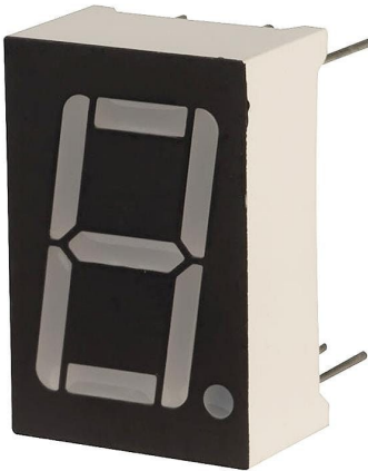
A seven-segment display shows one denary digit, often driven by BCD
