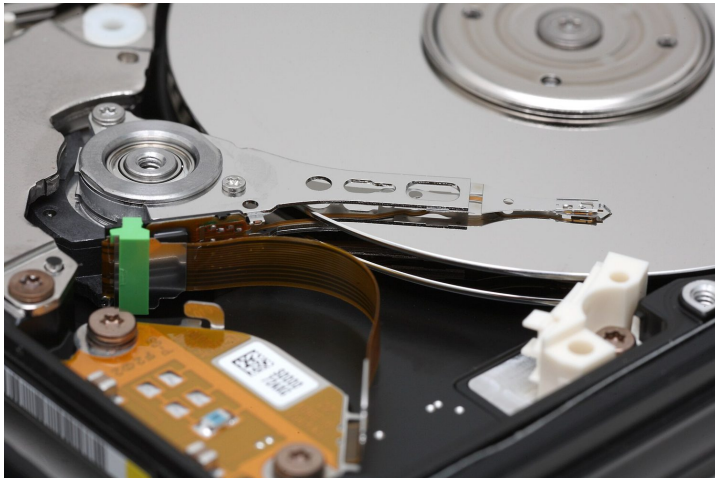
The physical storage the logical schema hides: a hard disk's spinning platters and read/write head
