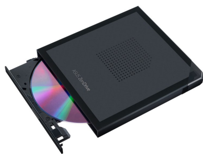
An optical disc drive: a laser reads tiny pits on a CD, DVD or Blu-ray disc
