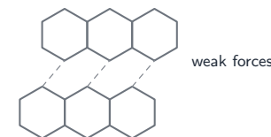
graphite layers slide; spare electrons let it conduct
