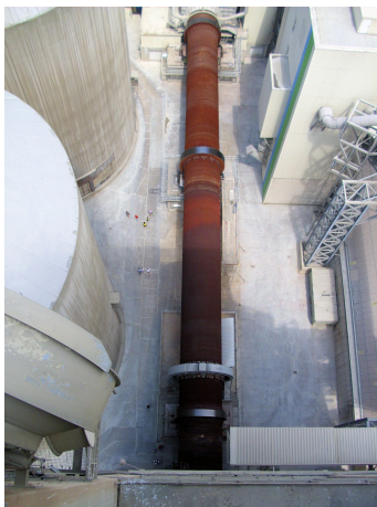
Heating limestone (calcium carbonate) in a kiln decomposes it to calcium oxide — a thermal decomposition
