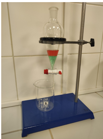
A separating funnel splits two immiscible layers — how the organic product is recovered from the reaction mixture
