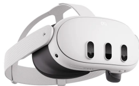
A virtual reality headset: two small displays and motion sensors track the head
