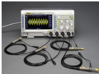
A real oscilloscope: the grid lets you read off the period and the amplitude
