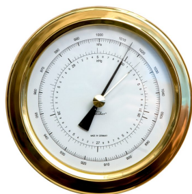
A precision aneroid barometer measures atmospheric pressure
