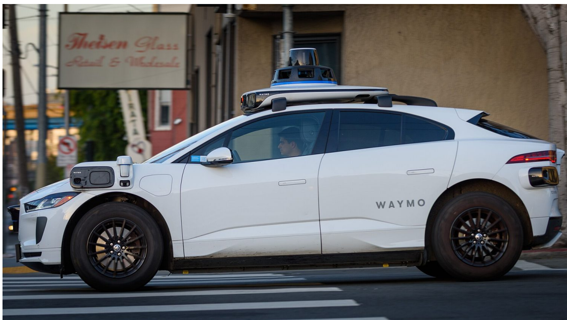
A self-driving car: sensors on the car let a computer steer it with no driver
