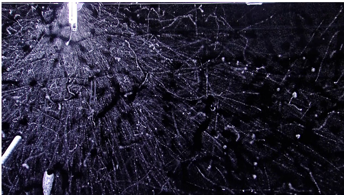
Each beta particle from the source leaves a thin track in a cloud chamber – direct evidence of separate, random decays
